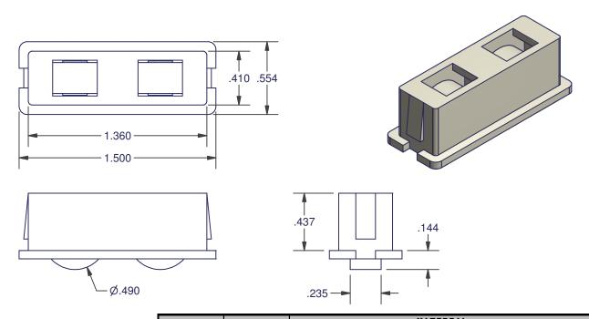
MATERIAL **AMESBURY** REFERENCE ITEM # ITEM # HOUSING **ROLLER AXLE** 400340 26-1000 NYLON NATURAL CELCON STAINLESS STEEL
